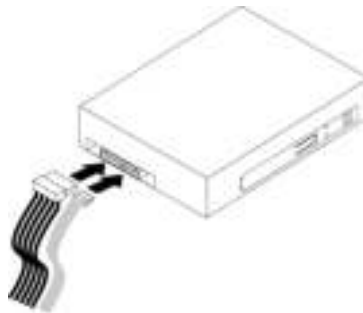
Figure 33. Connecting the cables to the rear of the new optical drive
