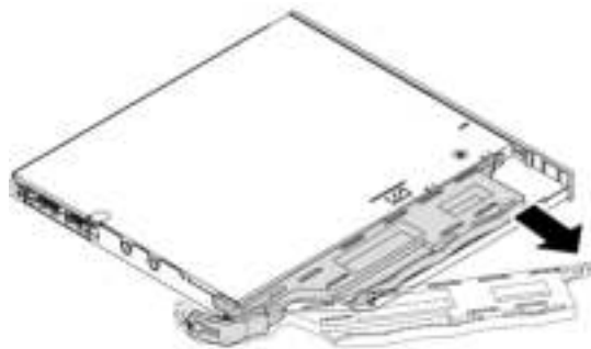
Figure 49. Removing the bracket from the slim optical drive
