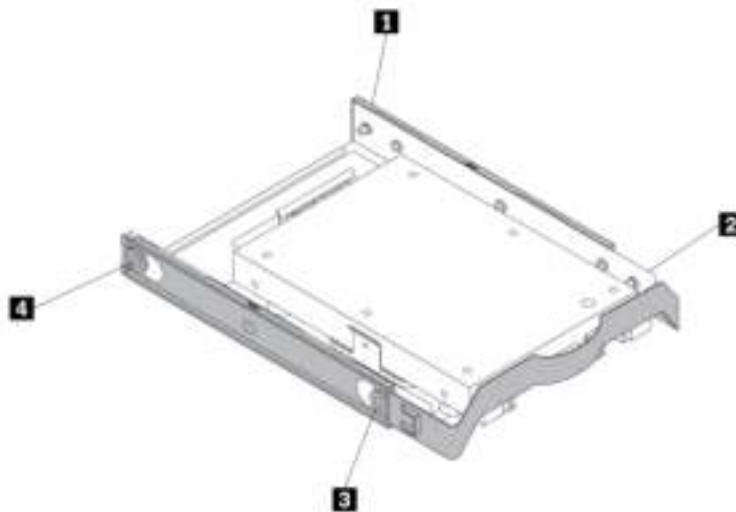
Figure 87. Installing the storage-drive converter together with the 2.5-inch storage drive into the storage-drive bracket
