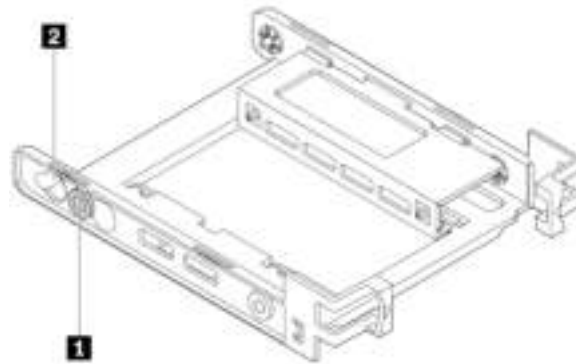
Figure 58. Removing the pin and installing it into the new slot
